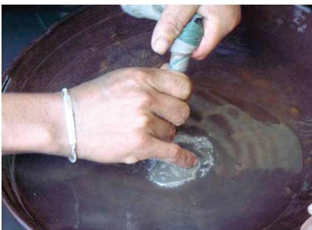
Mercury is used in many South American gold mines. The silvery mercury is mixed with the ore, then boiled off, leaving pure gold—and serious environmental issues.
