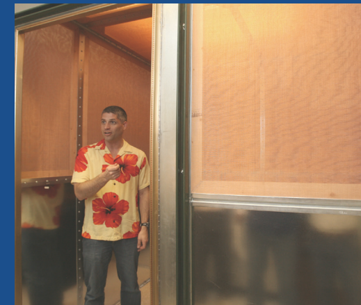
Paul Kieffaber, assistant professor of psychology, shows off one of the Faraday chambers in the department's EEG lab. "We have two different booths where we can run," Kieffaber said. "We just pop them in a chair, put a cap on their heads and start recording their brain waves." The Faraday chambers provide isolation from "noise" coming from lights and electrical sources.
