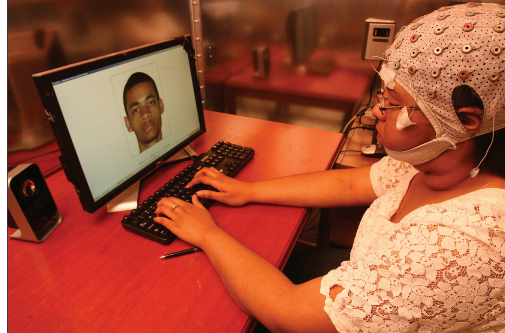
Inside the ISC's Faraday cage, Aline Roberts views a series of target faces of various races, each shown for half a second. Her reactions to each face are monitored by EEG. The cage isolates the subjects from data-polluting "noise" generated by the electric fields of the building's lights, wiring and appliances.
