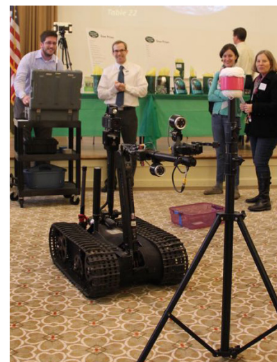
Interactive demonstrations of technology filled the room at the Teaching & Technology Expo. In this picture, a participant is guiding a bomb disposal robot to place the "bomb" (yarn) in the "safe zone" (purple container). The robot, once used in the military but now retired, is used to teach robotics in the K-12 school systems.
